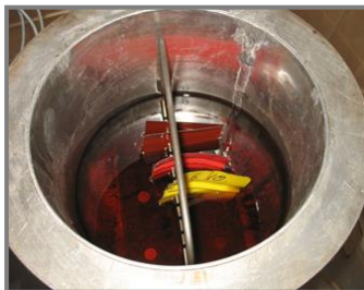
Internal coating fuel resistance test
